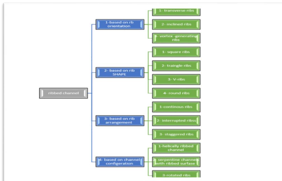
Fig. 2. Classification of ribbed channel: The schematic was designed and prepared by the authors to illustrate the geometry used in the study.
