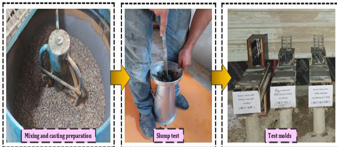
Fig. 5. Stages of material mixing, slump testing, and casting specimens in the laboratory.
