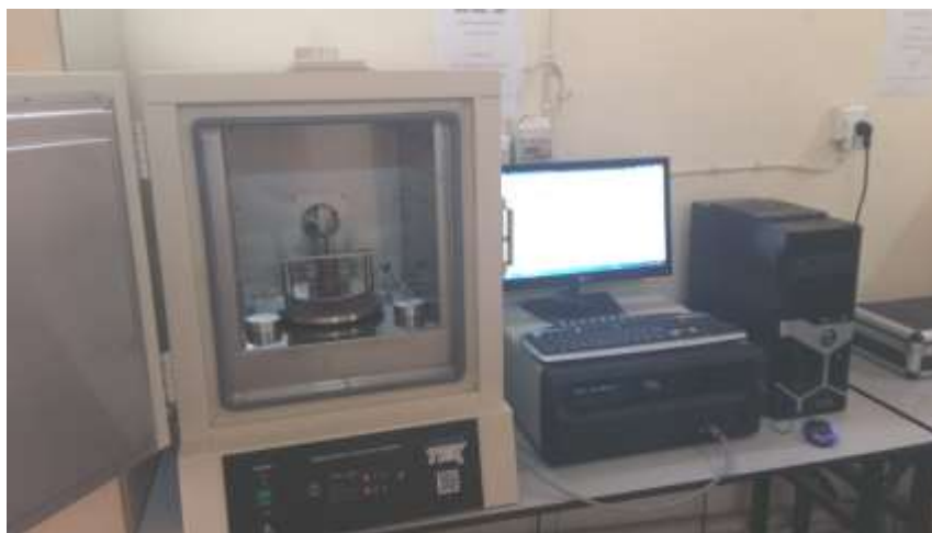
Fig. (3) Thermal constant analyzer (Hot Disk) with samples
