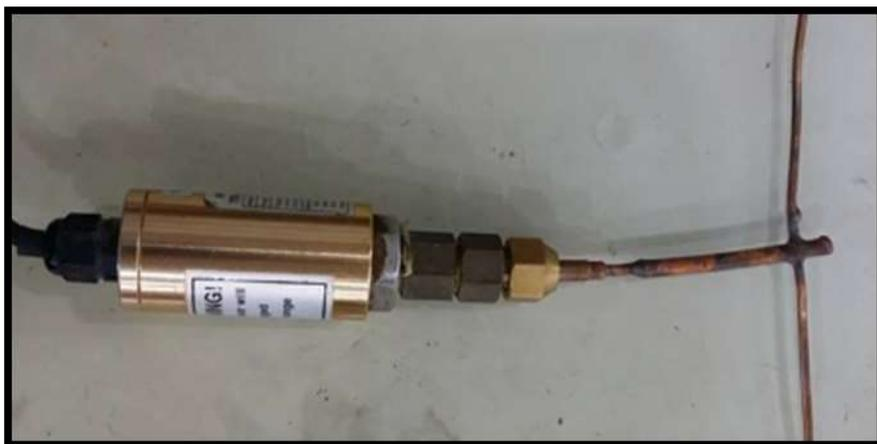
Figure (2): T-connection of pressure sensor to the capillary tube
