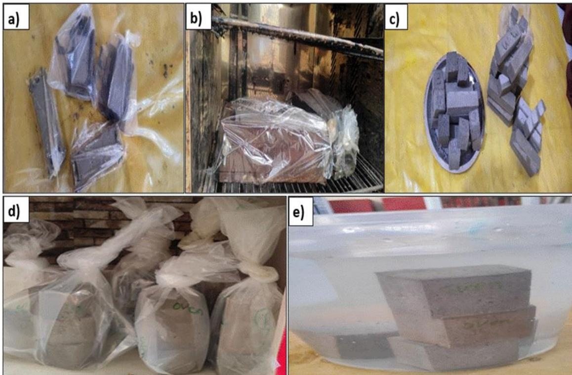
Fig. 3. Curing Regimes, a) Sealed molds at ambient temperature, b) Sealed molds in oven at 80°C, c) Demolded sample, d) Sealed cured sample at ambient temperature after demolding, e) Cured sample in water after demolding.
