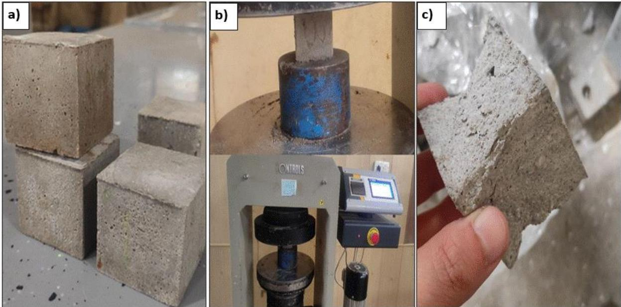
Fig. 6. Compressive Strength test, a) The test sample, b) Compressive strength test machine, c) Tested sample.
