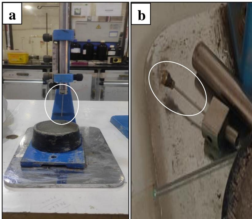
Fig. 5. Setting time test, a) initial, b) final.
