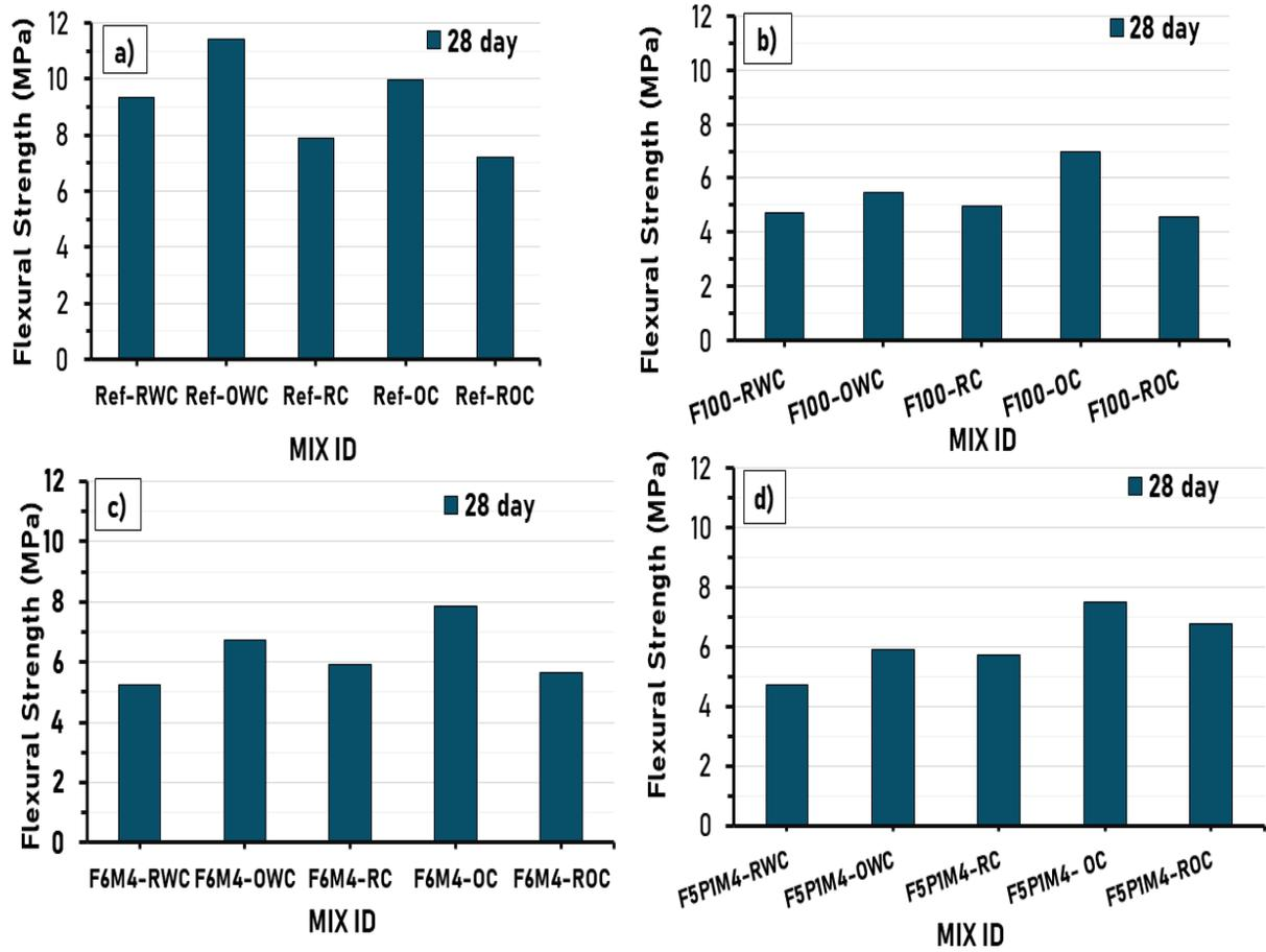
Fig. 11. Flexural strength test results of mortars at 28 days in different curing regimes: a) Reference, b) Mix F100, c) Mix F6M4, d) Mix F5P1M4.
