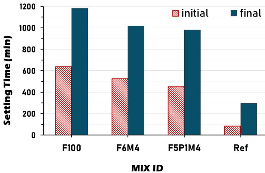
Fig. 9. Initial and final setting time results of alkali-activated mortars.
