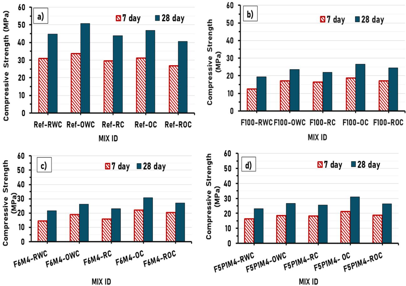
Fig. 10. 7- and 28-days compressive strength test results of Geopolymer and reference mortars in different curing regimes: a) Reference mixes, b) Mix F100, c) Mix F6M4, d) Mix F5P1M4.
