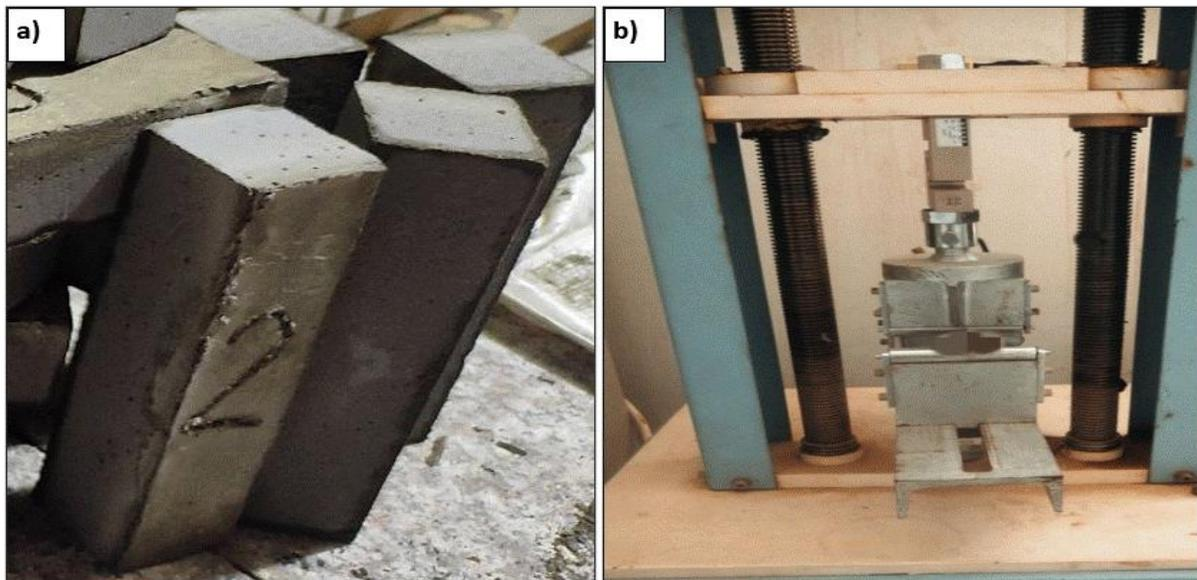
Fig. 7. Flexural strength test. a) The test sample, b) Flexural strength test machine.
