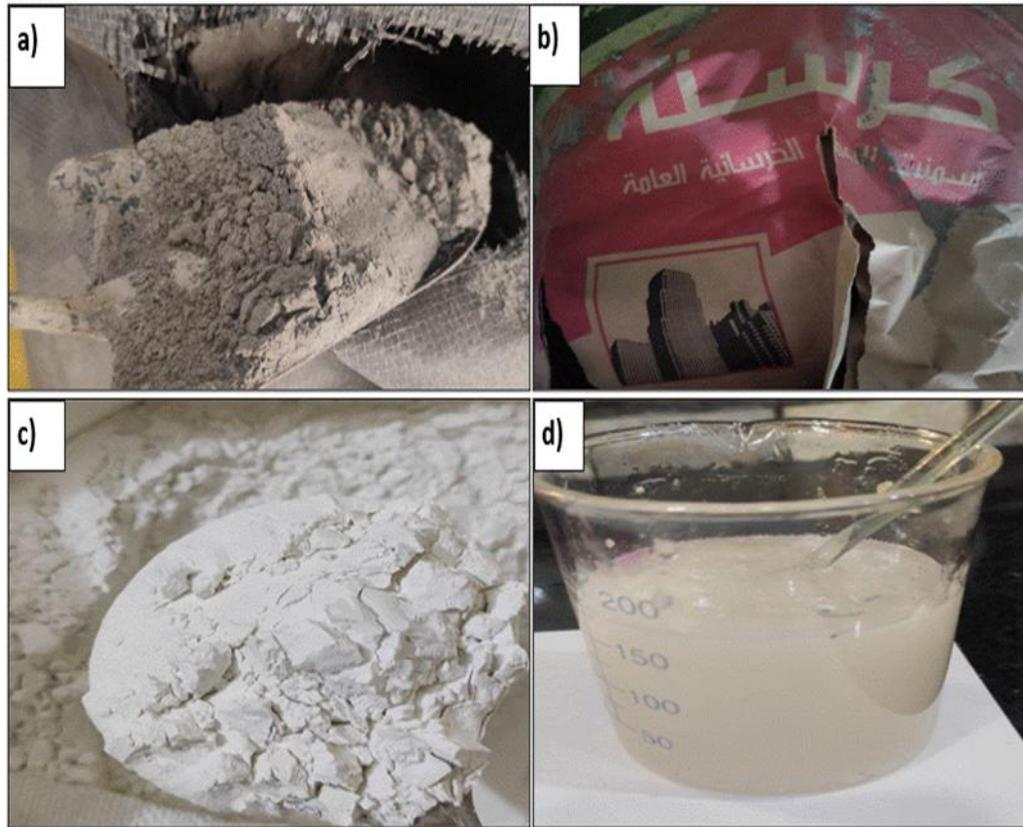
Fig. 1. The materials that used in this study a) Fly ash, b) Ordinary Portland cement, c) metakaolin, d) SS activator.
