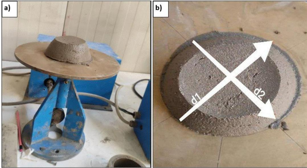
Fig. 4. Flow test of mortars a) Apparatus of flow test, b) The examined sample.
