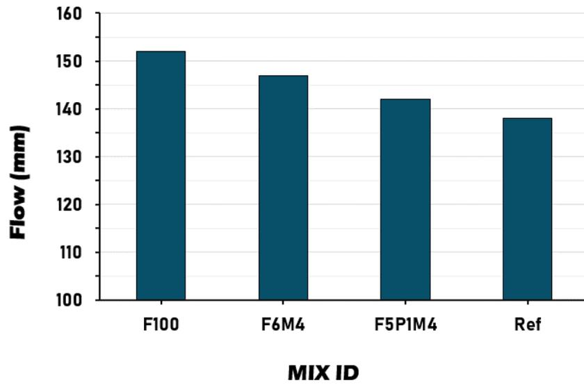
Fig. 8. Flow test results of mortar.
