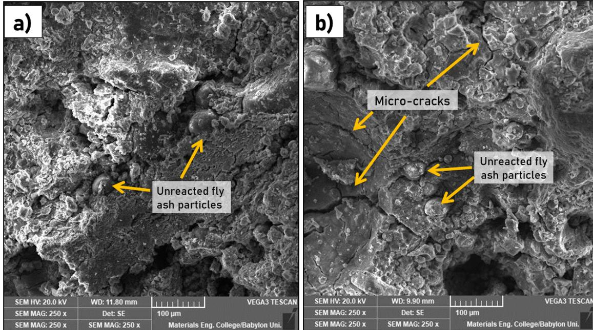
Fig. 12. SEM analysis test results of oven cured mortars at 28-day age a) Mix F6M4, b) Mix F100.
