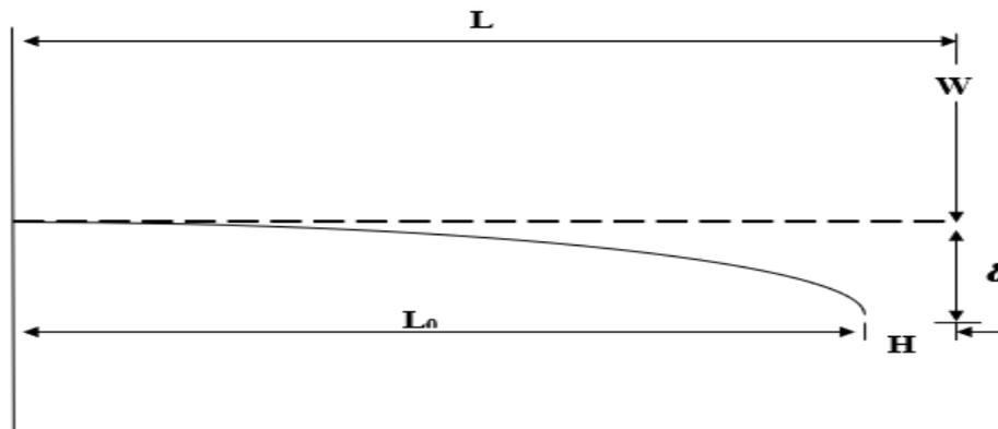
Fig (A-2):-Schematic representation of curvature of the cantilever
