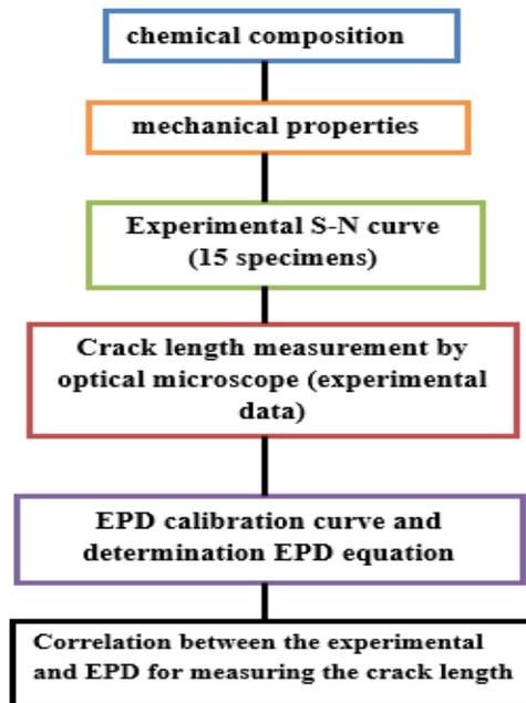
Fig (4) Flow chart of the experimental work
