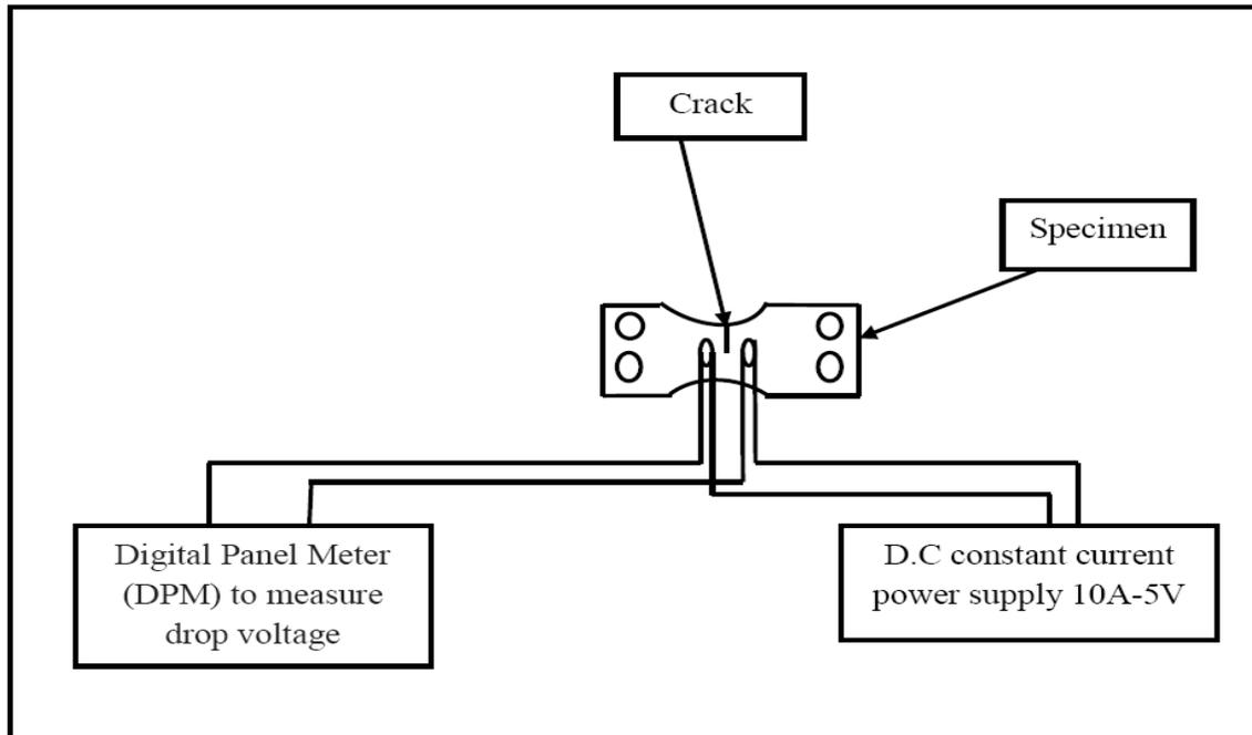
Fig (2) Schematic diagram of EPD circuit
