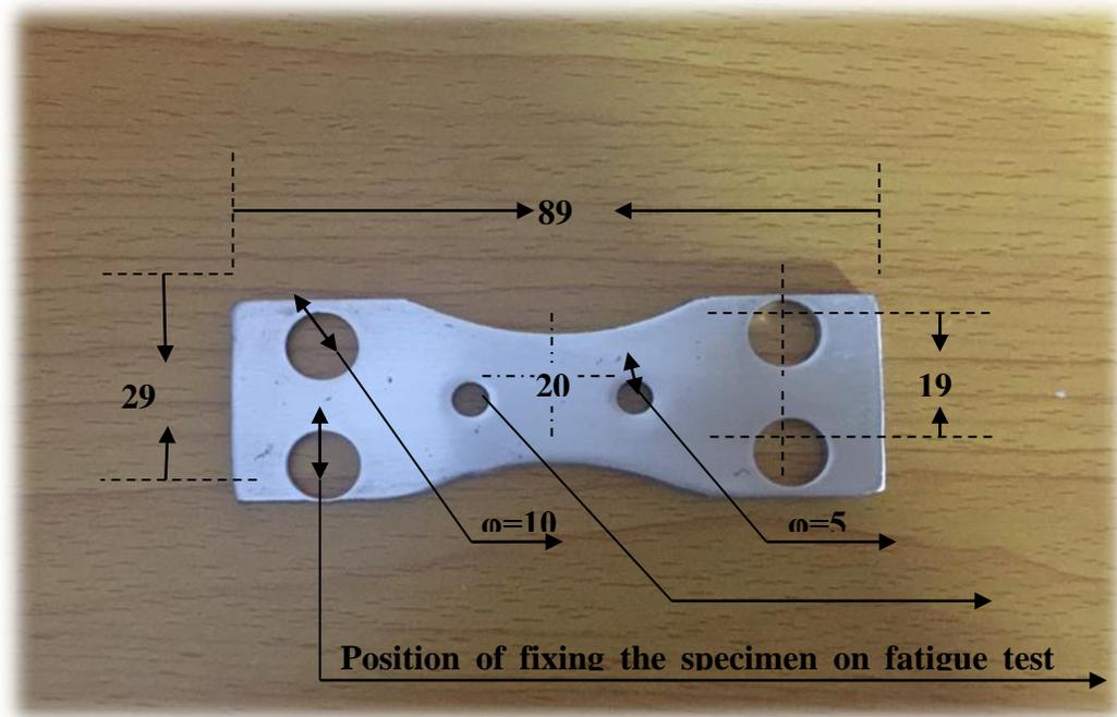
Fig (3) Reverse cyclic bending fatigue test specimen of 3mm constant thickness (all dimensions in mm) according to ASTM D3479M-96 standard.
