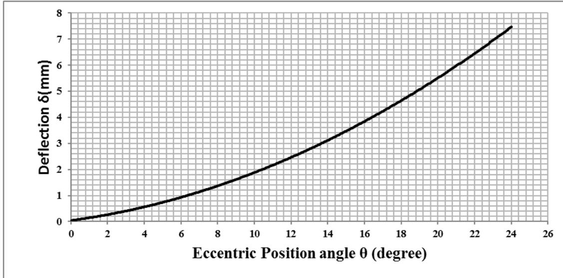
Fig (A-3): Calibration curve between bending deflection and eccentric position angle of AVERY machine for aluminum alloy
