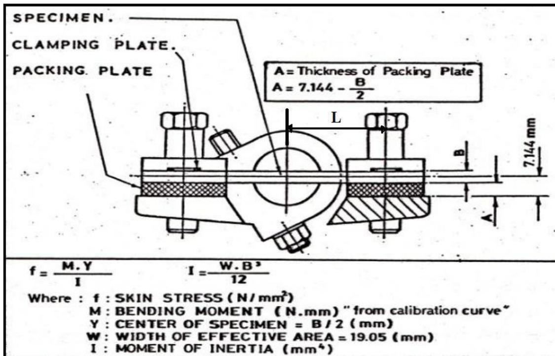
Fig (A-1): Schematic representation of fixing method, and how to calculate maximum bending moment
