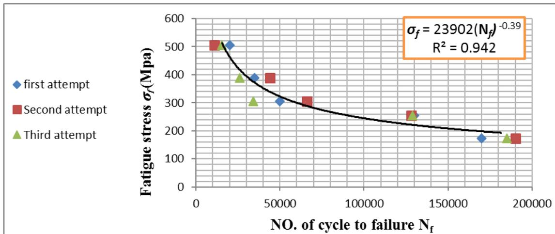
Fig (6) Relationship between applied stress and No. of cycle to failure ( $N_f$ )
