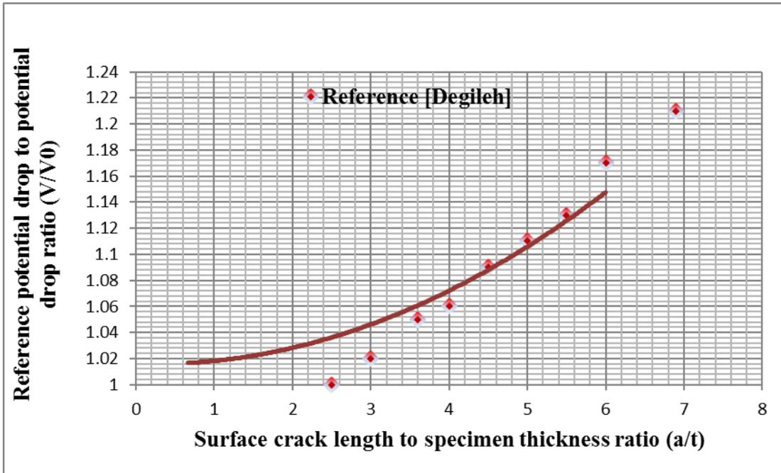
Fig (8) Comparison between calibration curve in this work and other in reference [Degeilh]
