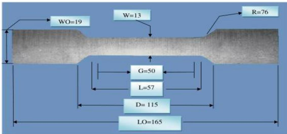
Fig (5) Standard tensile test specimen
