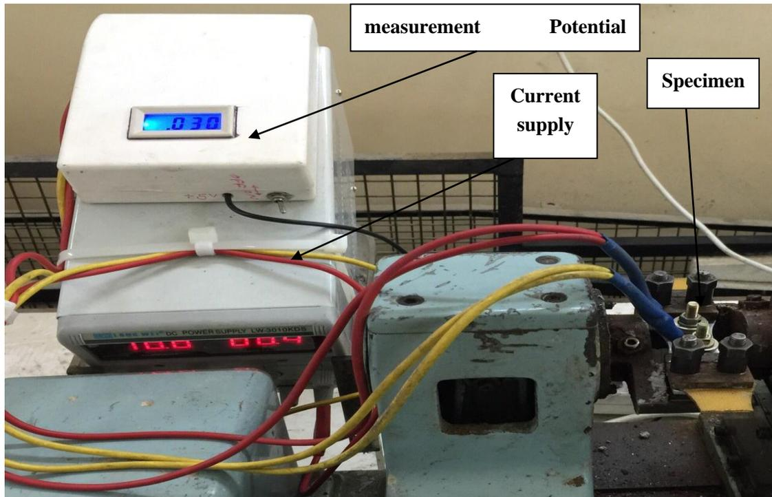
Fig (1) Potential drop system fixed on fatigue specimen
