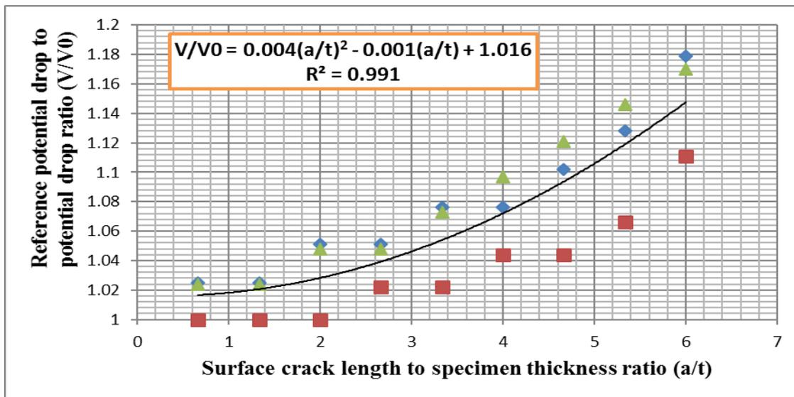
Figure (7) Experimental calibration curves
