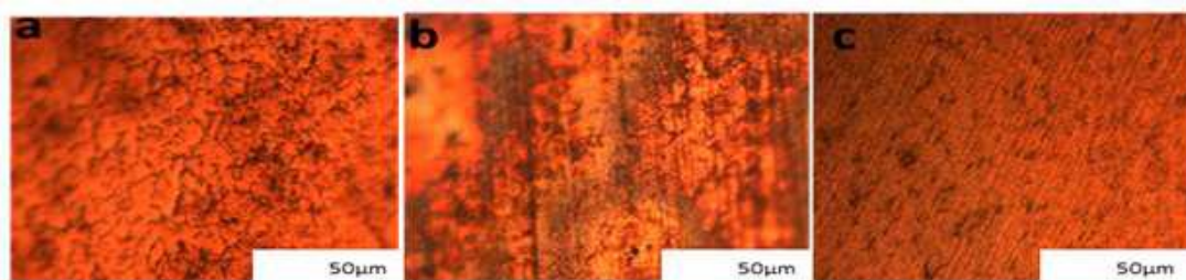
Fig. 18. Quenching specimens in coconut water of 30, 45 and 60 min respectively. [Peter et al, 2018]
