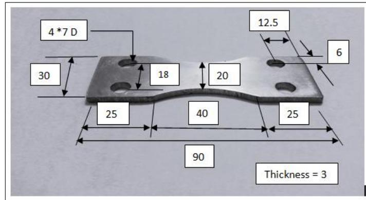
Fig.1. Sample of the fatigue specimen corresponds with the din 50133 standard requirement.
