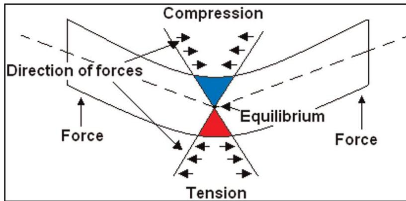
Fig. 8. The graph shows how the stress is distributed throughout the material as it is bent (Shukla PP, Swanson PT, Page CJ, 2014).
