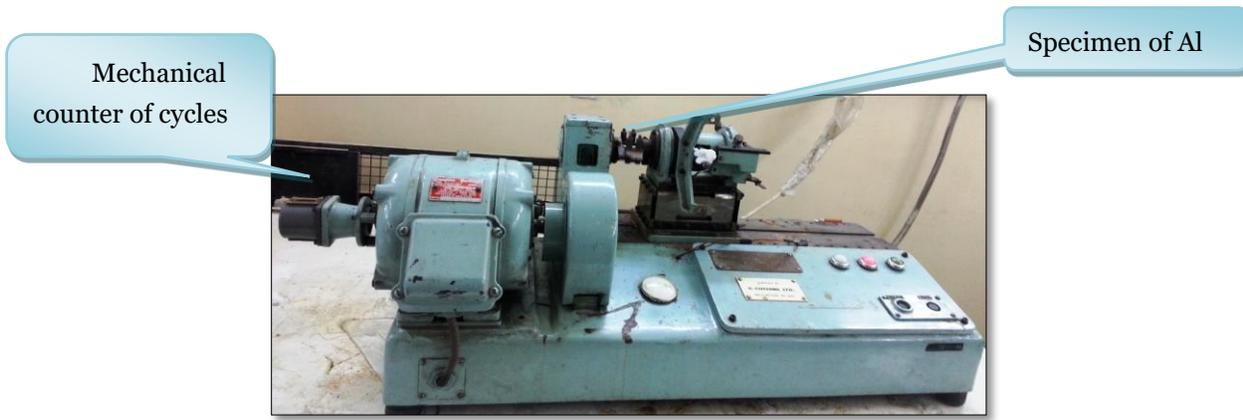
Fig.2. Bending machine for fatigue.
