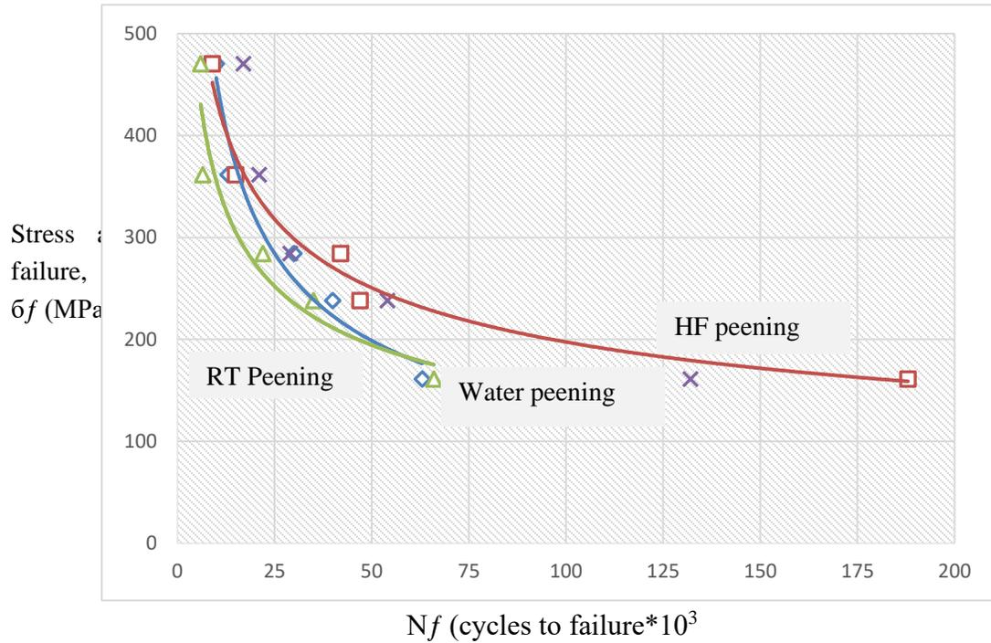
Fig. 7. S-N Curves for laser shock peening and unpeened processes using HF acid and clean water under constant load.
