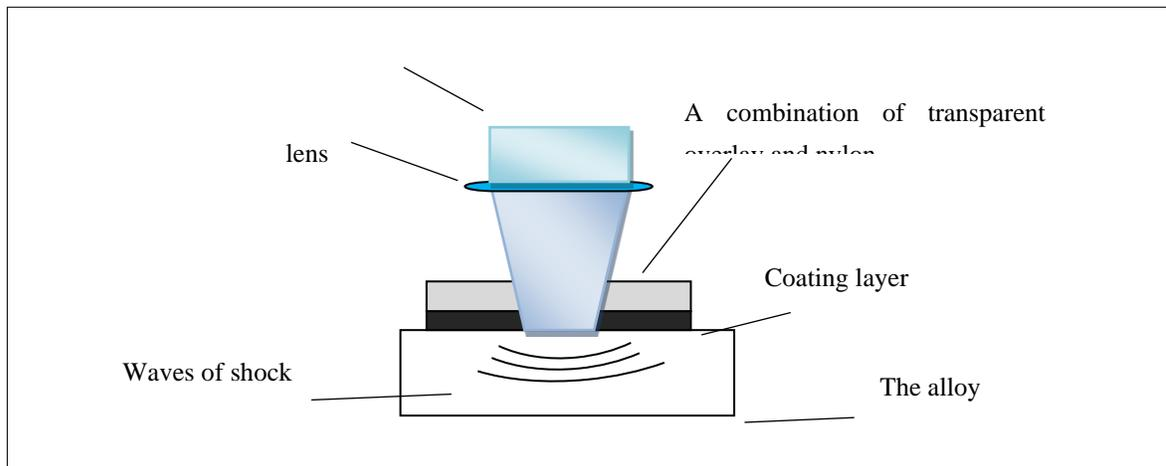
Fig.3. The essential idea of laser shock peening.
