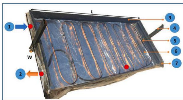
Fig. 2. experimental design of collector: (1) inlet -tank 1; (2) outlet - tank 2; (3) collector enclosure; (4) angle guide rod; (5) serpentine absorber tube; (6) fiberglass insulation; (7) plastic cover.
