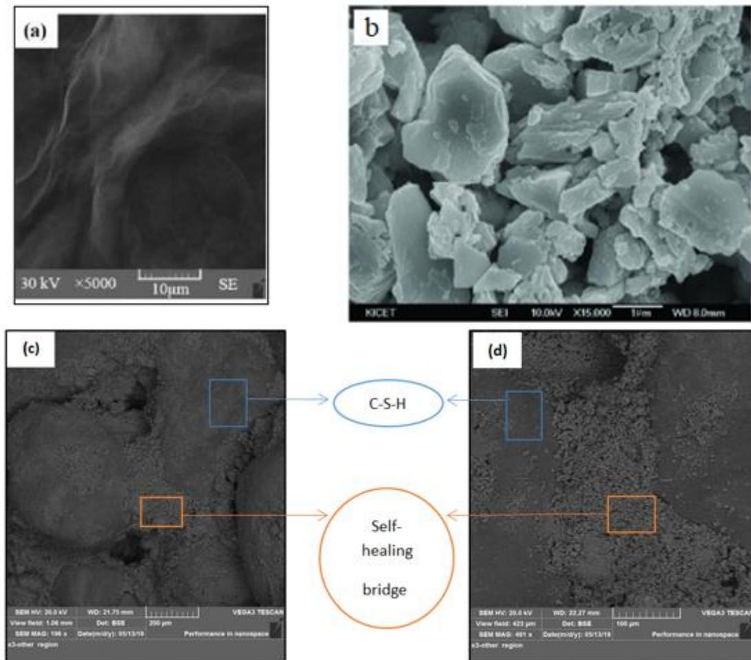
Fig. 9. (a) SEM of base mortar, (b) SEM of cement powder, (c) & (d) SEM for bio-mortar with (5ml) Nutrient broth Proteus.
