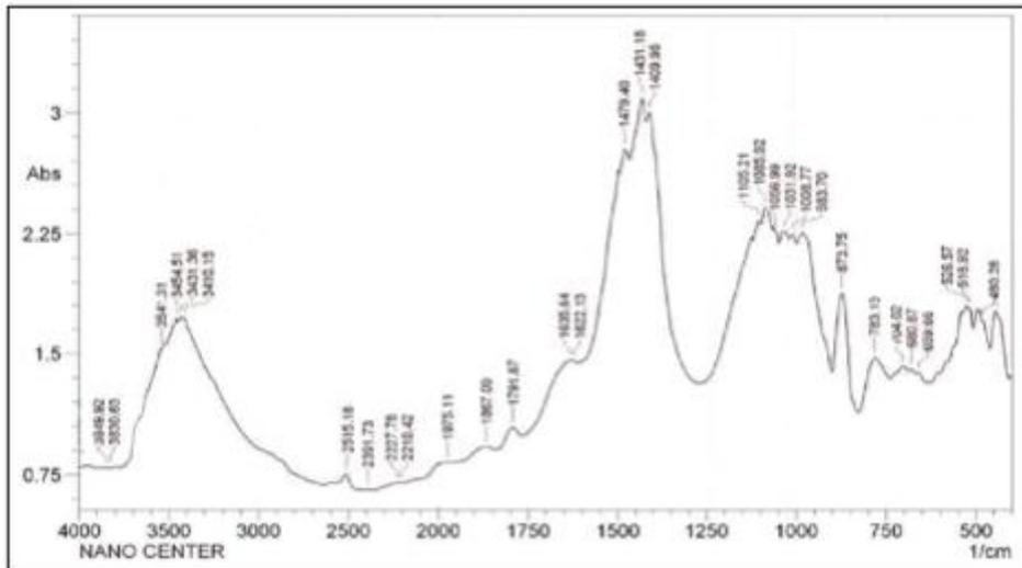
Fig. 6. FTIR test for bio-mortar with (25 ml) of Nutrient broth E.coli bacteria.
