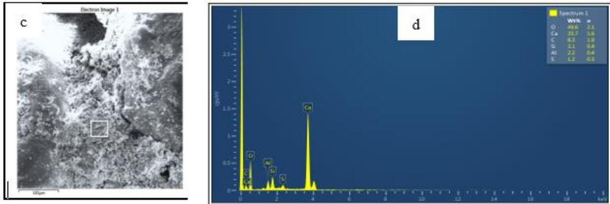
Fig.8. (a, c) SEM for bio-mortar with (5ml) Nutrient broth Proteus. (b,d) EDX for bio- mortar with (5ml) Nutrient broth Proteus.
