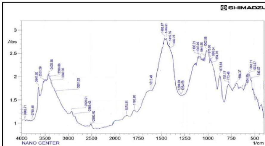
Fig.7. FTIR test for bio-mortar with (25ml) of Nutrient broth Proteus bacteria.
