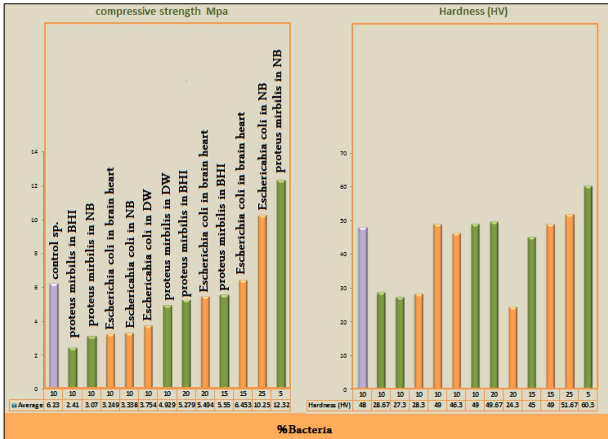
Fig. 3. Compressive strength for bio-(N-type) mortar. Fig. 4. Hardness test for bio-(N-type) mortar.
