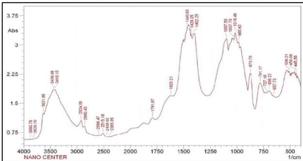
Fig. 5. FTIR spectrum of cement mortar with 5ml of BHI E.Coli bacteria
