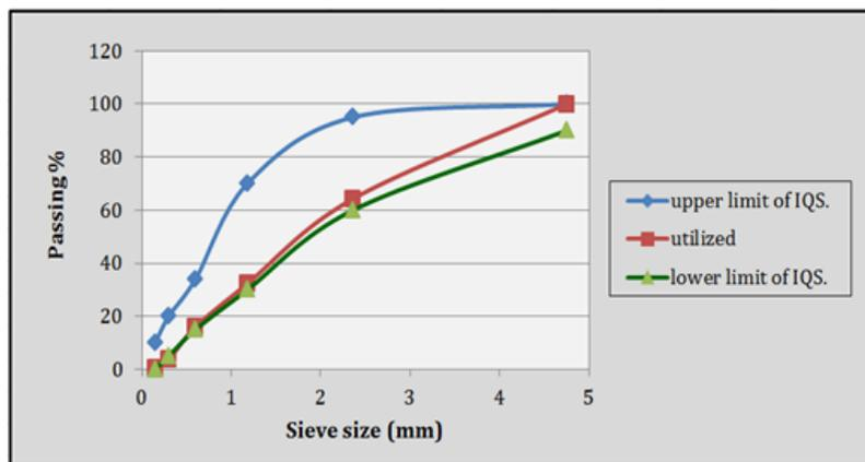
Fig.1. Grading of natural sand Iraqi Specifications Measurement...(1984/ 45).
