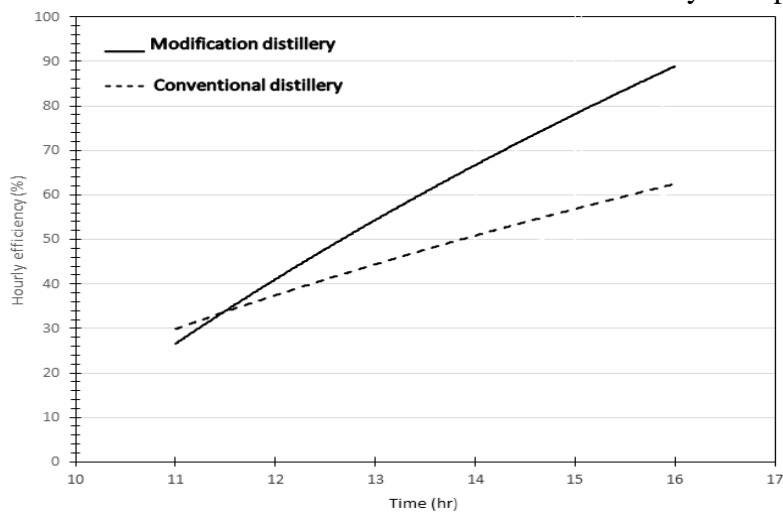
Fig. (21). Variation of hourly efficiency for the conventional and modified solar still on Jan. 17. 2018, Kirkuk, Iraq.
