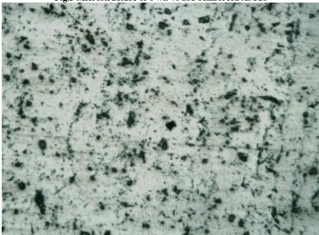
Fig.4 Microstructure of 9 wt. % SiC reinforced AMCs
