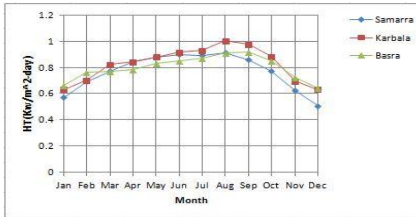
Fig. 16, monthly average, total daily radiation for PV panels inclined at (30 deg).
