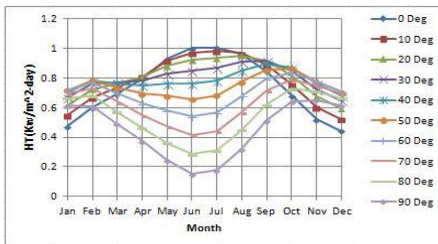
Fig. 15, monthly average, total daily radiation on inclined PV panels surface in Basra city.
