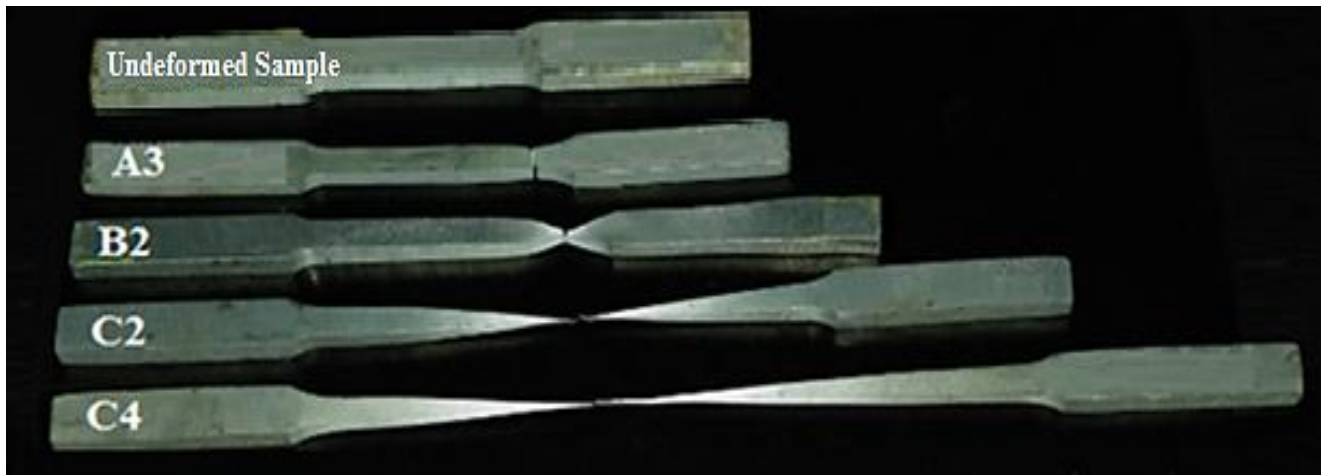
Fig. 1 Fracture of the tensile test samples
